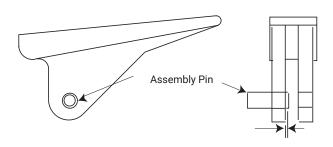
2.38 (.094) dia x 6.35 (.250) long Pin protrusion of approximately .38 (.015) seeks hole in PCB
